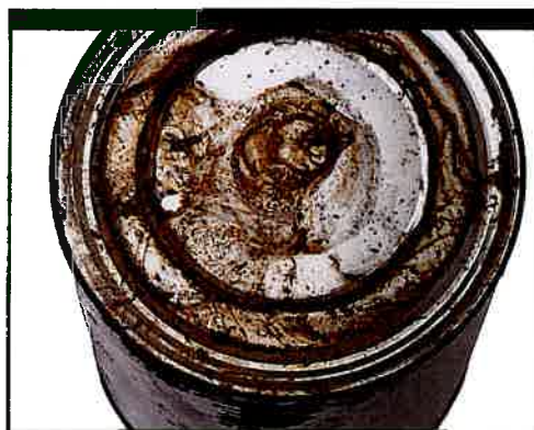
Rust that cannot be wiped off
