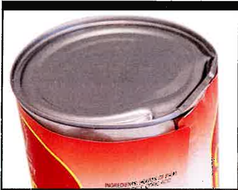
Severe dent in seam
